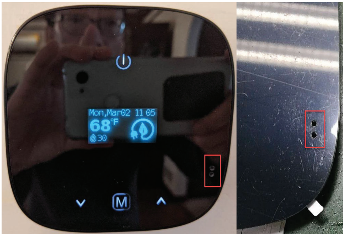
PC 面板上的开孔 (With the Red Rectangle Marking)
