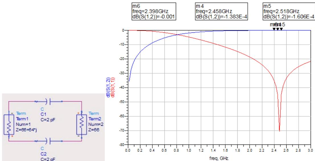
Finally, according to the  $S(1,1)$  and  $S(1,2)$ , the Term1  $66 + j64$  Ohm is well matched to the Term2 66 Ohm. C1 and C2 also works as the DC blocking capacitors which prevent the flow of DC signals into the following RF circuits.
