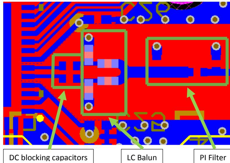
The DC blocking capacitors and LC Balun can be easily identified. The PI Filter is employed for harmonic reduction. However, you may already notice the layout is a little bit strange. We have this kind of strange layout, because we must use the distributed parameter models for the real-world microwave design. The layout, PCB stackup, stripline and microstrip impedance control, dielectric constant control become crucial [3].
