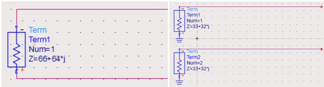
The CC2538 differential impedance is shown in the left-hand side of above diagrams. This impedance can also be described as the right-hand side diagram if the reference plane changes to ground and the coupling is omitted.
