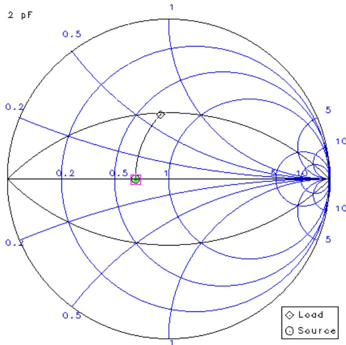
Place the 2pF capacitors on the each trace of the differential pair:
