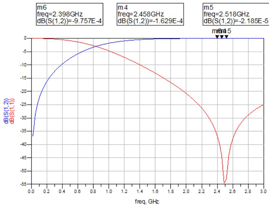
According to the S (1,1) and S (1,2), the Differential Ended 66 Ohm is well matched to the Single Ended 50 Ohm. The two inductors and two capacitors of the lumped LC Balun are L1, L2 and C3, C4
