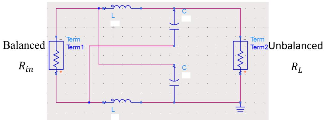
The characteristic impedance ( $Z_0$ ) of the lumped LC Balun is given by
